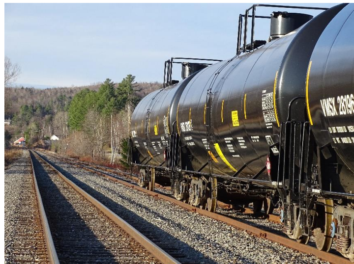
Propane cars for Superior Propane on SLR interchange with NHCR in N. Stratford, NH. New CWR on mainline. (SLR photo)
